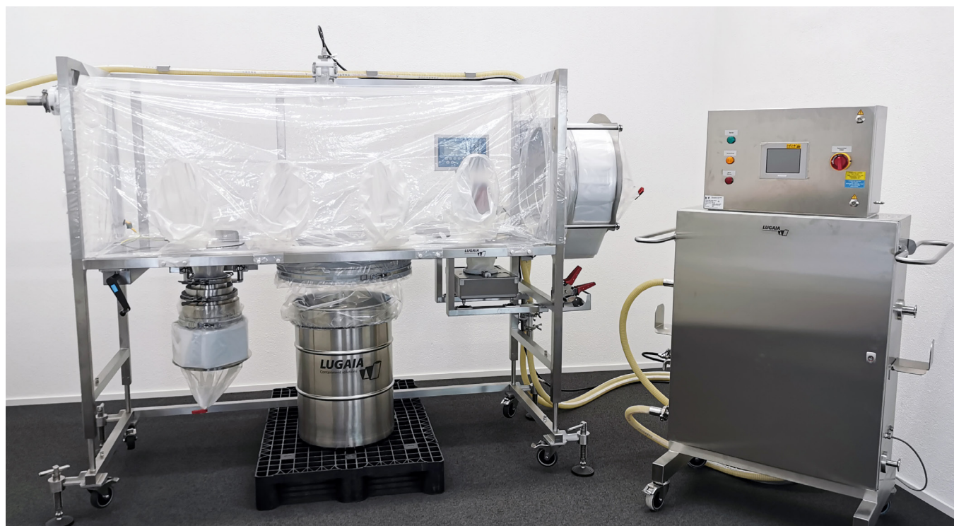
Complete flexible isolator system with a premium ventilation unit for stable pressure conditions and precise airflow control.
