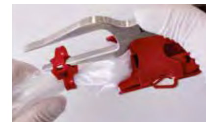
Loosen the cable tie cover
