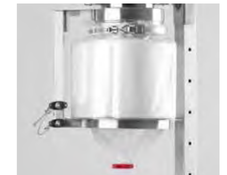
Continuous Liner System (CLS)
