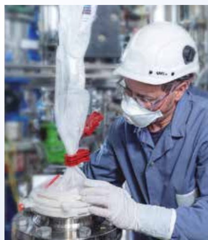
Closing the SafePort TransferBag using the SafeSeal System
