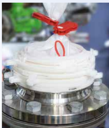
Separation of the SafePort TransferBag using the SafeSeal System
