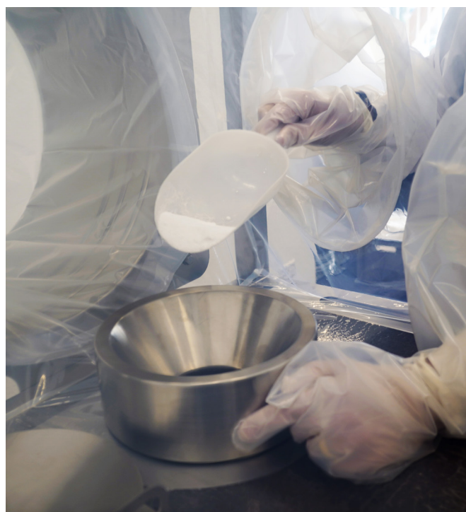
Powder handling in the Lugaia SafeFlex isolator
