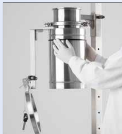
Fit the O-ring on the carrier tube
