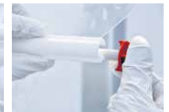
Remove round stick by pressing it out
