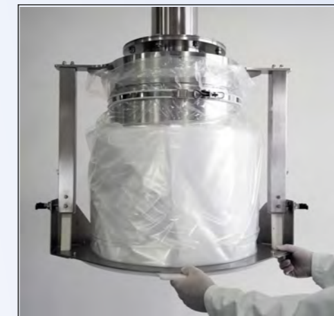
Pull the outermost fold over the liner support. Seal with clamping ring.
