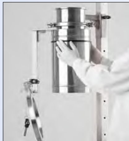
Fit the O-ring on the carrier tube
