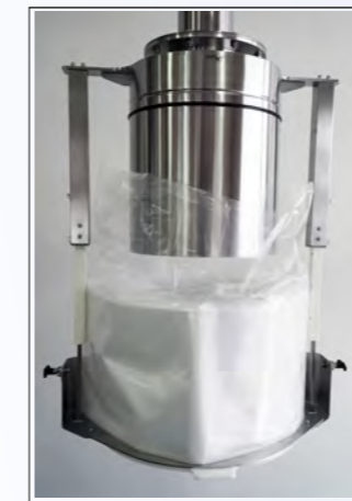
Fit the O-ring and position it in the lowest bead. Put the placement basket with liner unit on the telescopic rods.
