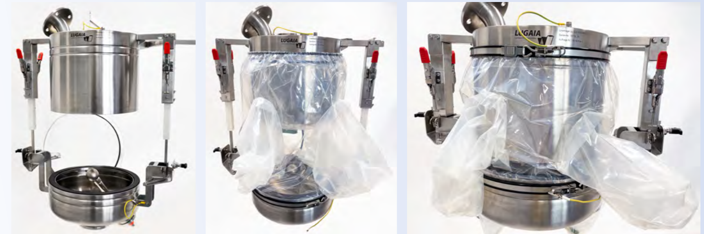
Liner carrier with washing hopper with integrated spray ball
