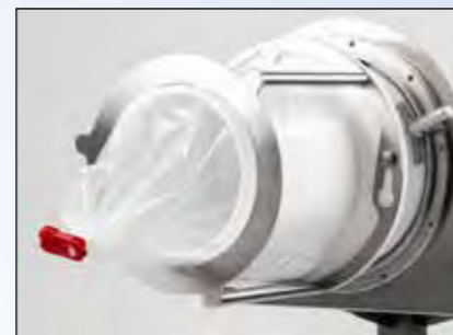
Close the Continuous Liner with SafeSeal
