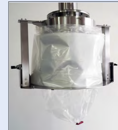
Push the telescopic rods evenly upwards. Close with the SafeSeal Closure System.
