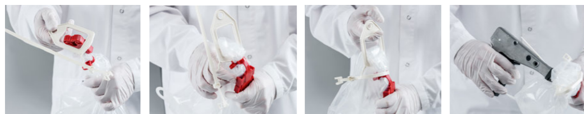
Slip the hanging tool on Bend the foil Put on cable ties Tighten cable ties
