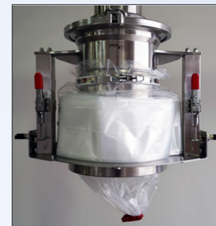
Continuous liner fully loaded and ready for filling
