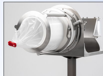
Close the Continuous Liner with SafeSeal
