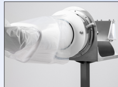
Put on the Continuous Liner
