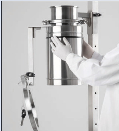
Liner carrier getting prepared for loading
