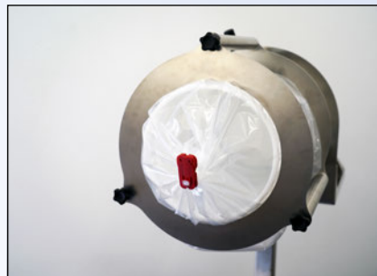
Close the Continuous Liner with SafeSeal
