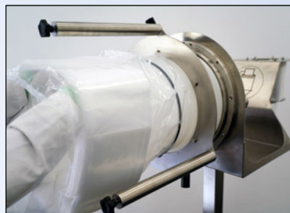
Put on the Continuous Liner
