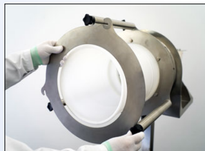
Remove the retaining plate
