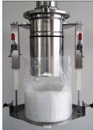
Liner carrier with mounting aid getting prepared for loading
