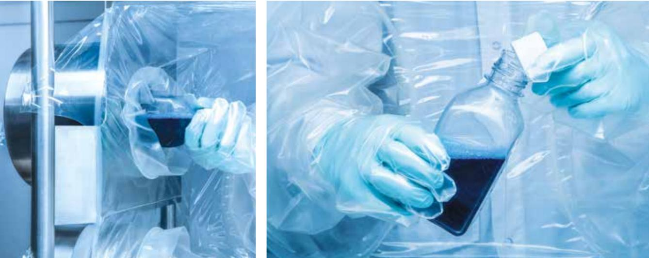
Isolators are used to protect the environment or the processed product. A very well-planned flexible containment isolator comes very close to a stainless-steel isolator in terms of protection and can offer various advantages depending on the application.
